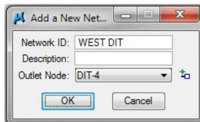
**NOTE:** The **Outlet Node** may be selected via the dropdown or by clicking **ID Outlet** and selecting the Node in the plan view.
