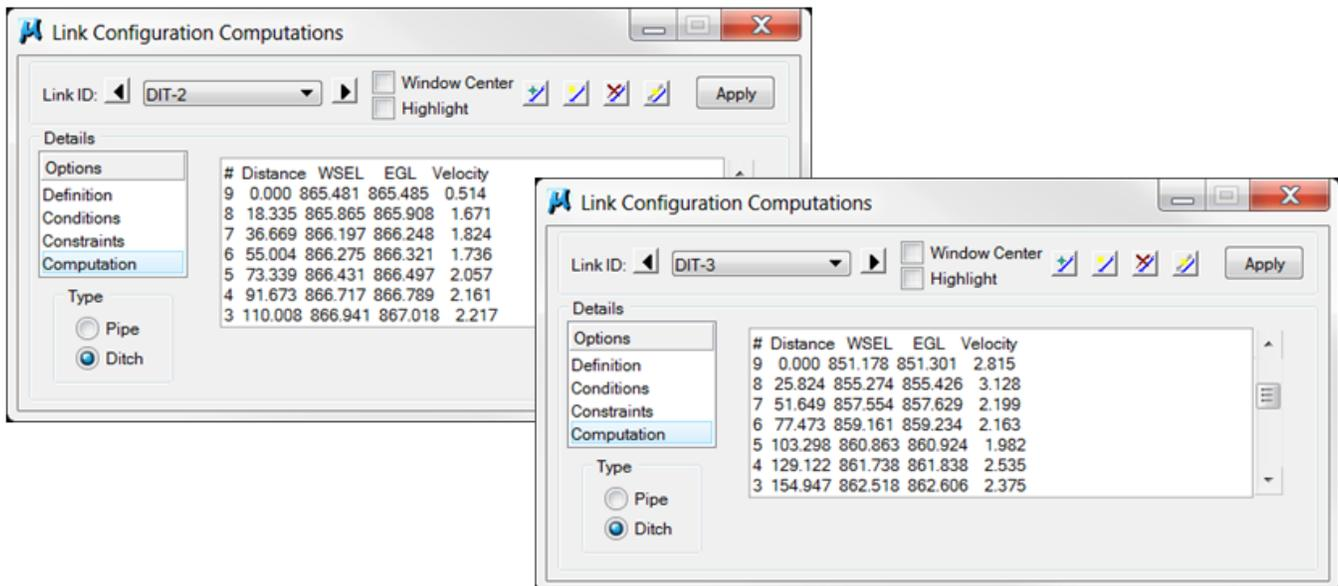
Using this information, we can determine if the existing conditions are adequate to convey the water along the fill line and critical points where more capacity may be required.
